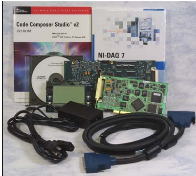
EVM320VC5509A + Keypad/display Module + Power Supply + Code Composer Studio + National Instruments PCI Card and Power Measurement Software Utility
