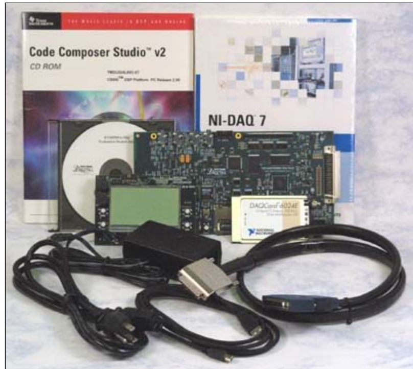
EVM320VC5509A + Keypad/display Module + Power Supply + National Instruments PCMCIA Card and Power Monitor Software Utility
