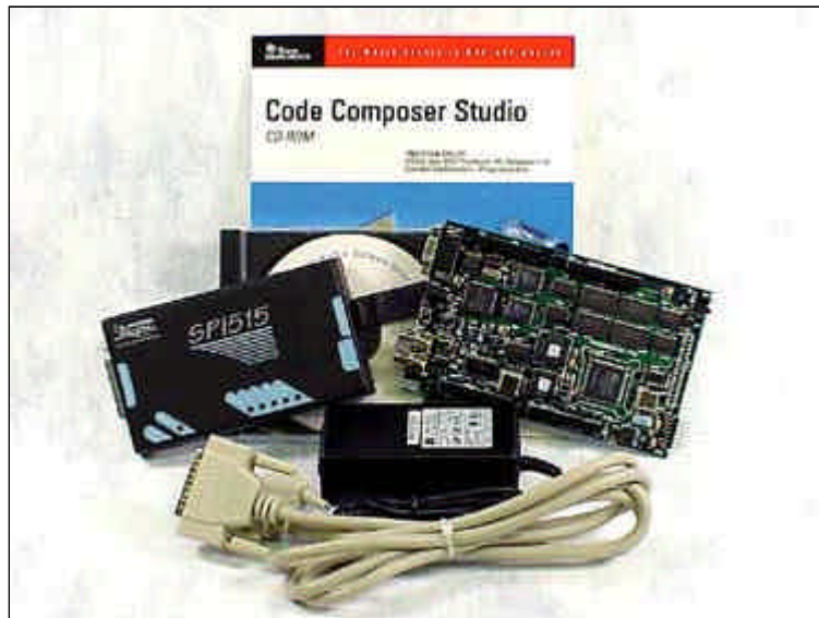
EVM320VC5410 + Power Supply + SPI515 JTAG Emulator + Code Composer Studio for the C5xxx
