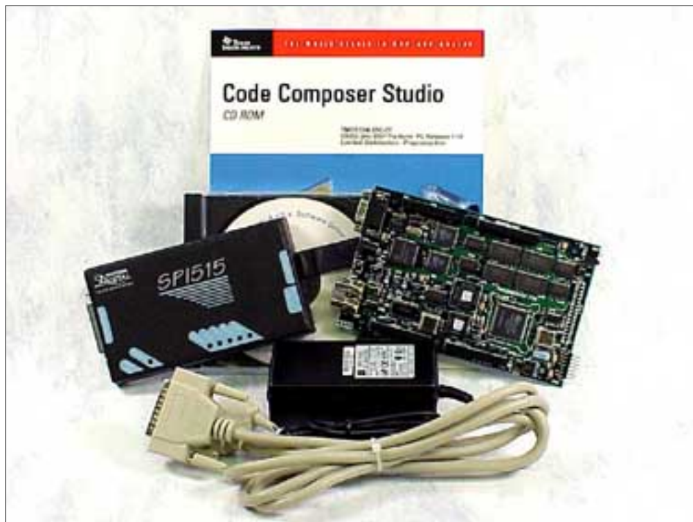
TMS320VC5402 Development System with Code Composer Studio
