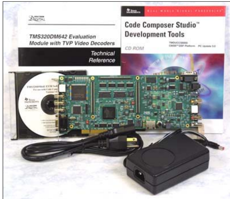
DM642 (720 Mhz, TVP Video Decoders) Evaluation Module + Power Supply + XDS510 USB Emulator + Code Composer Studio for C6xxx
