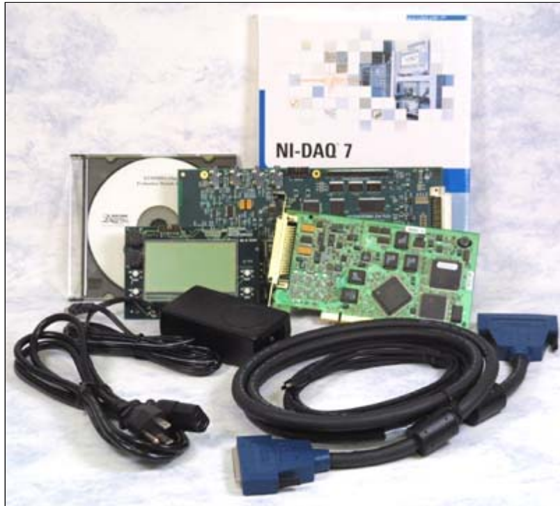
EVM320VC5509A + Keypad/display Module + Power Supply + National Instruments PCI Card and Power Monitor Software Utility
