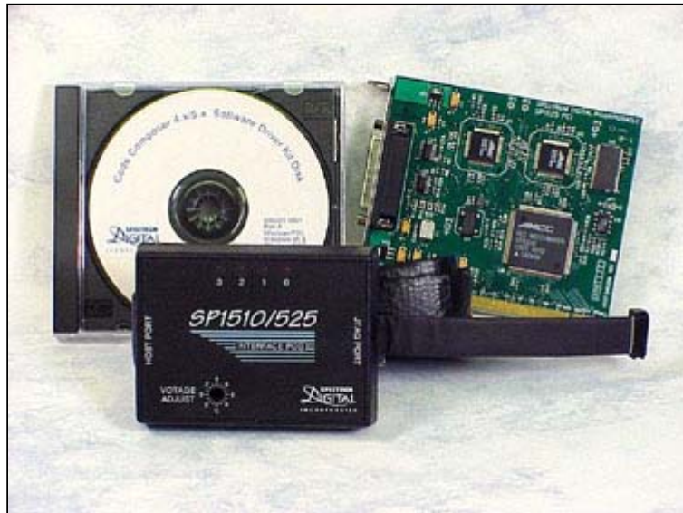
SPI510 ISA JTAG Emulator with Adjustable Voltage Pod and Code Composer Studio for TMS320C5xxx
